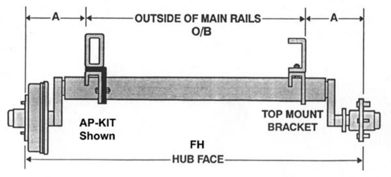
If you have difficulty measuring HUB FACE, you can measure dimensions O/B and A. HUB FACE = O/B + A + A.
